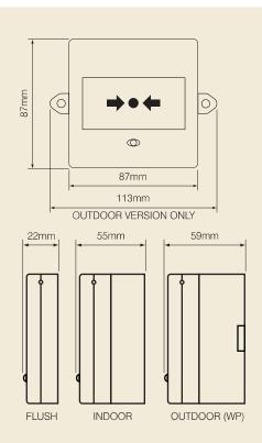
The CXL Universal Call Point combines a number of features into one package, simplifying selection and reducing stock variants. Designed to provide the facilities most frequently used, the Universal is the easy answer for the majority of conventional installations.
