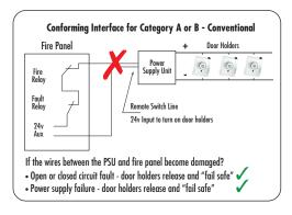
A 24V signal is used to control the PSU using the fire panel fire and fault relay.
